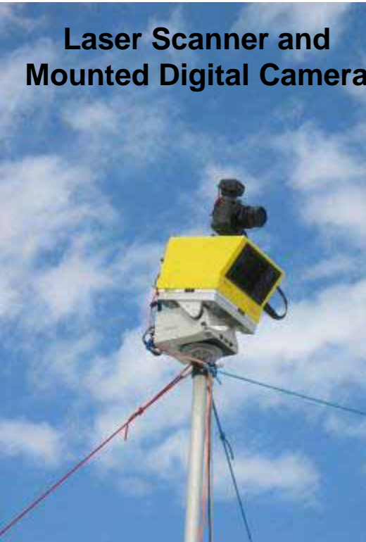
Setup to Scan Breakwater Harborside
