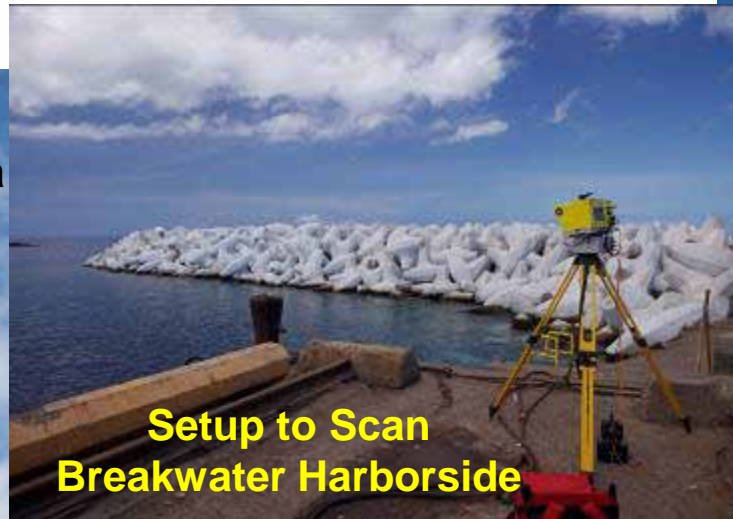
Laser Scanner and Mounted Digital Camera
